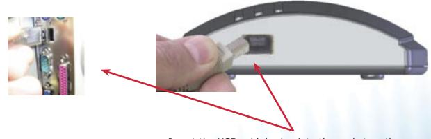
Insert the USB cable's plug into the socket on the rear of the HZ1500USB Adapter, then insert the other end into an available USB port on your computer.
